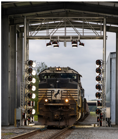
The digital train inspection portal uses AI and machine vision to identify mechanical defects in moving trains.
