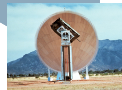
GTRI designed and built what was at the time the world's largest outdoor compact range at Fort Huachuca, AZ.
