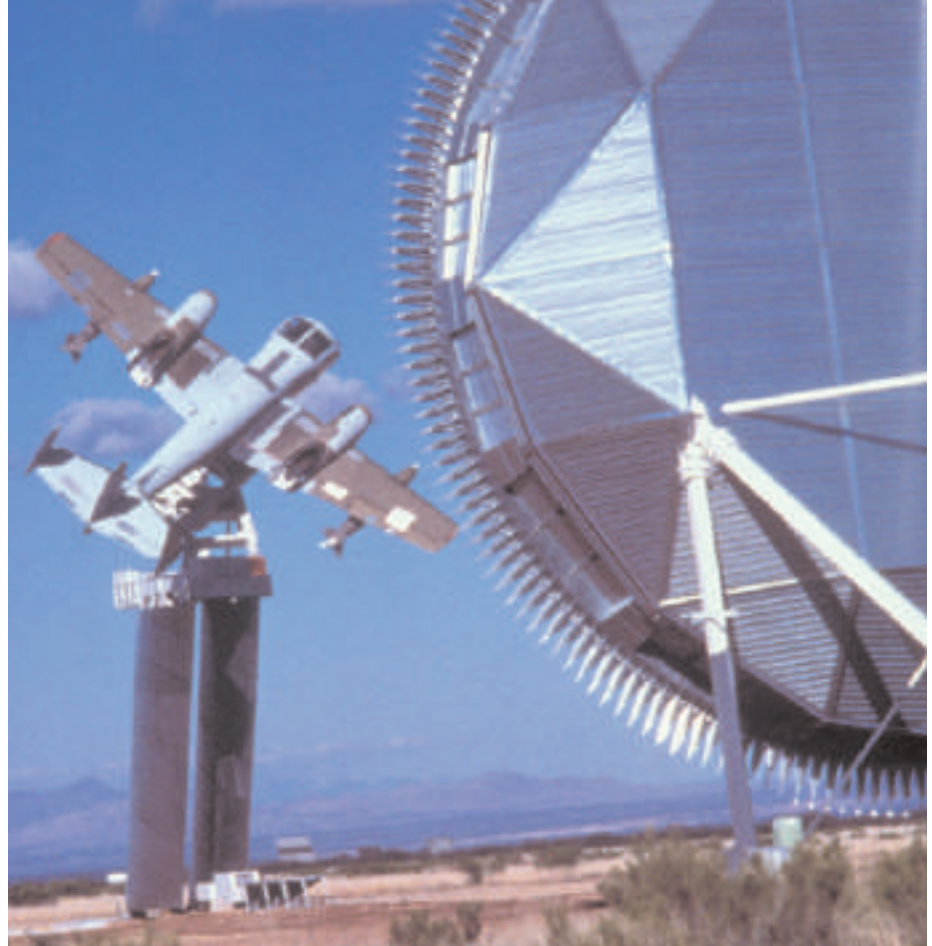
At Fort Huachuca, Arizona, the U.S. Army constructed an outdoor compact radar range thought to be the world's largest. GTRI scientist Dr. Richard C. Johnson invented the compact range in the late 1960s.
