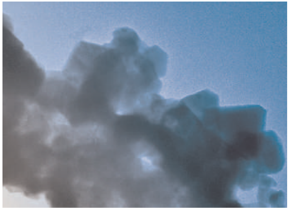
This transmission electron microscope image shows the copper branches of a 3-D foam structure that is part of an improved electrode developed by Georgia Tech researchers.
