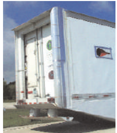
Aerodynamic improvements such as rounded corners, coupled with pneumatic controls for blowing air from slots, help reduce drag at the rear of heavy trucks.
