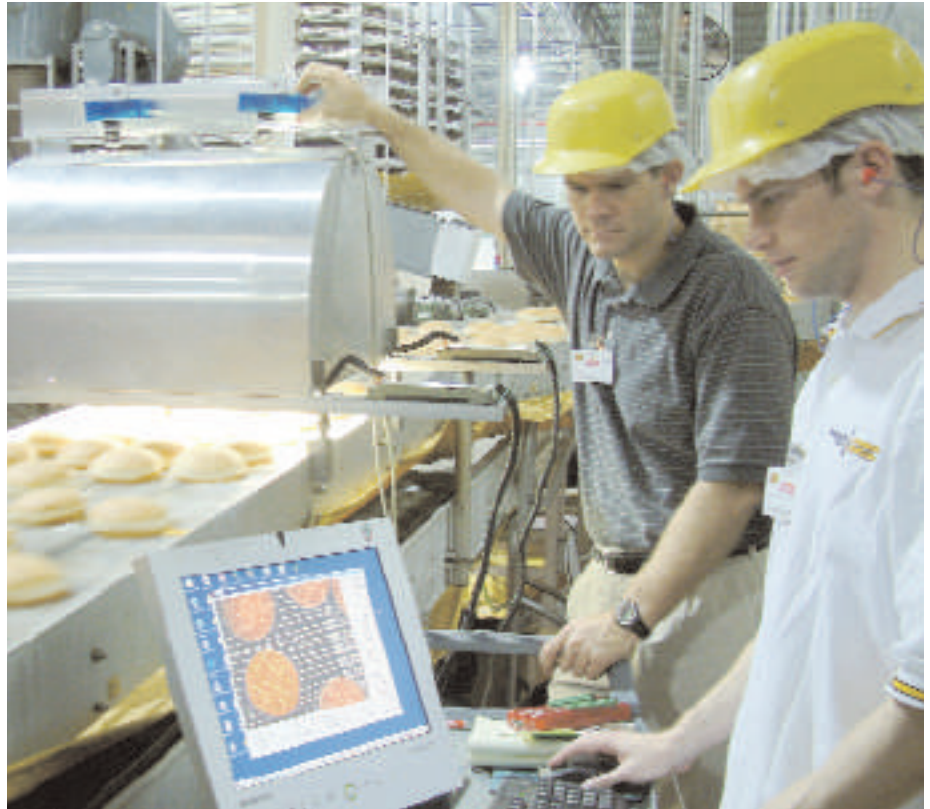
An automated product-inspection prototype is under development by Georgia Tech researchers working with Flowers Bakery in Villa Rica, Georgia. Researchers are introducing continuous imaging technology to the large-scale production of sandwich buns.
