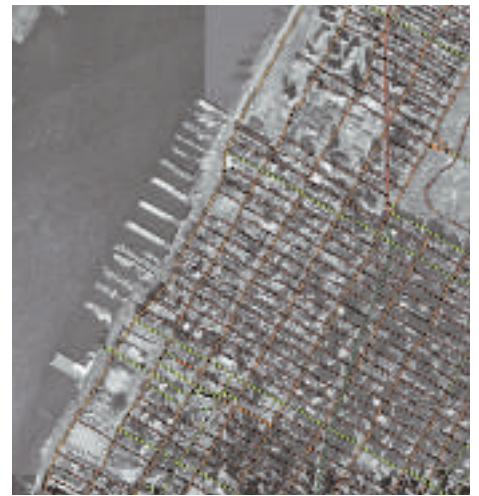
U.S. Geological Survey satellite imagery is overlaid with U.S. Department of Transportation street data in Manhattan in this FalconView-generated map.
